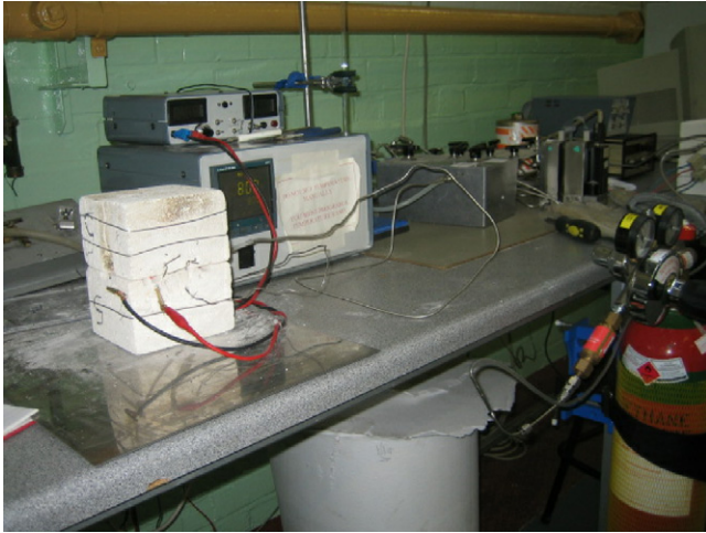
Fig. 3. Temperature cycling test system for Adelan small tubular cells.
