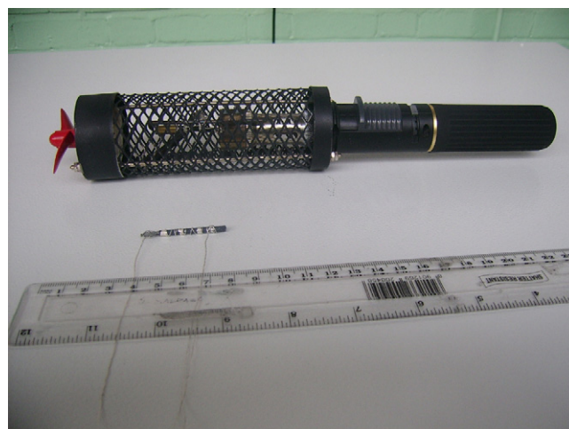
Fig. 2. Adelan tubular SOFC and hand held demonstration device that powers a fan.
